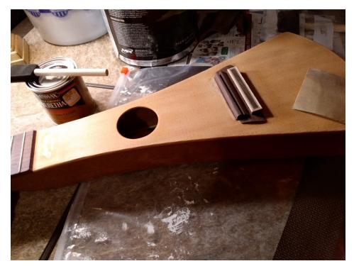
7. The top of the bridge saddle groove, the saddle and the nut all sanded down about 1mm to achieve standard classical guitar string action height.
