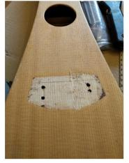
3. Prepared surfaces and glued new bridge to guitar.
